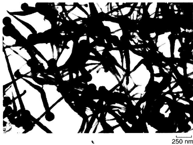
Fig. 3 Condensate obtained from the vapours liberated by a \text{CaGa}_2\text{O}_4/\text{CaCO}_3/\text{C} mixture in Ar at 1800^\circ\text{C} .
