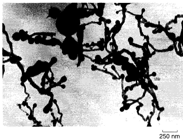
Fig. 4 Condensate obtained from the vapours liberated by a Al 2 O 3 /B/Ga 2 O 3 mixture in H 2 at 1800 °C.
